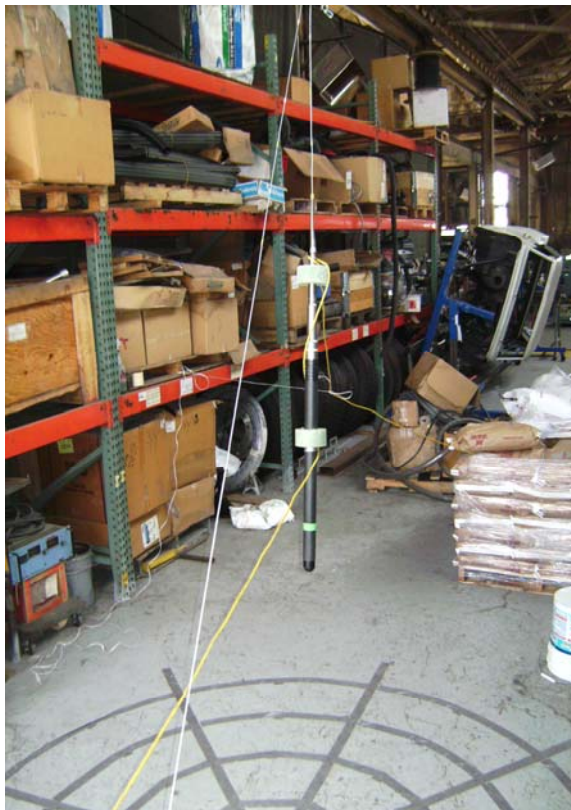
#3B: Gamma-ray sonde with Styrofoam centralizers
