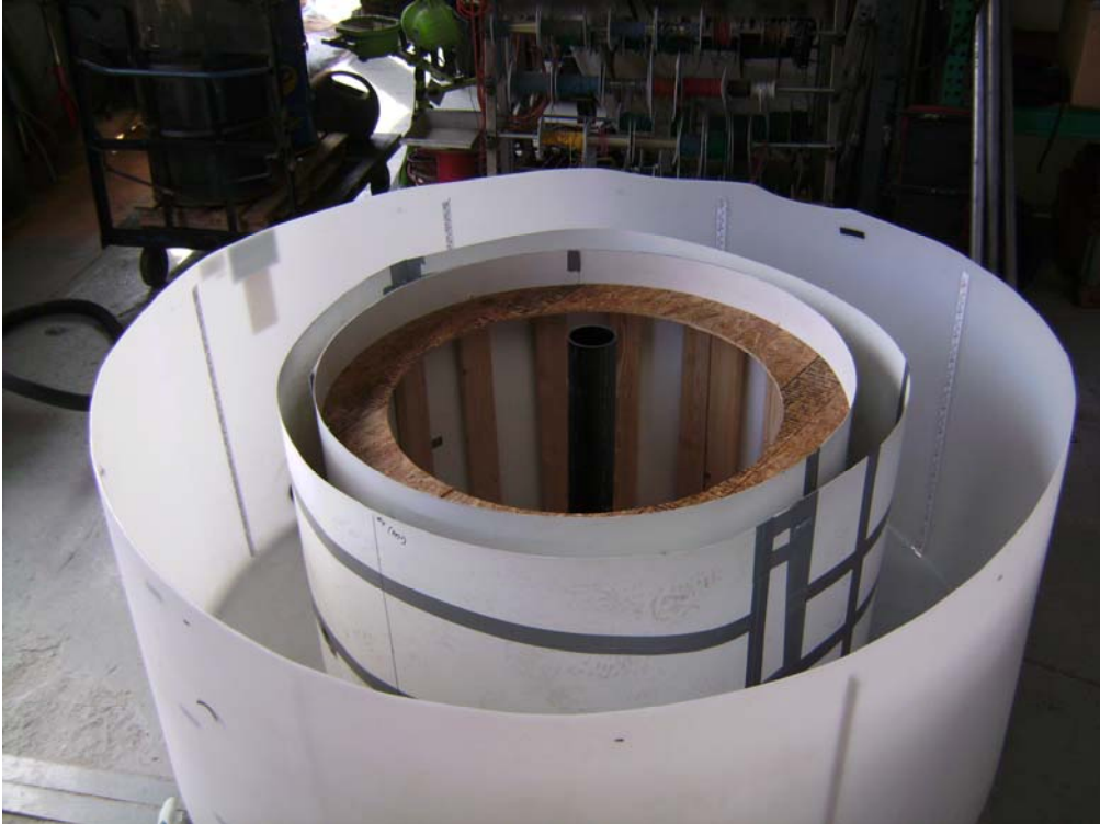
Figure #4A: Test tank set up for radial depth of investigation tests showing plywood forms and nested cylinders, prior to filling with product.
