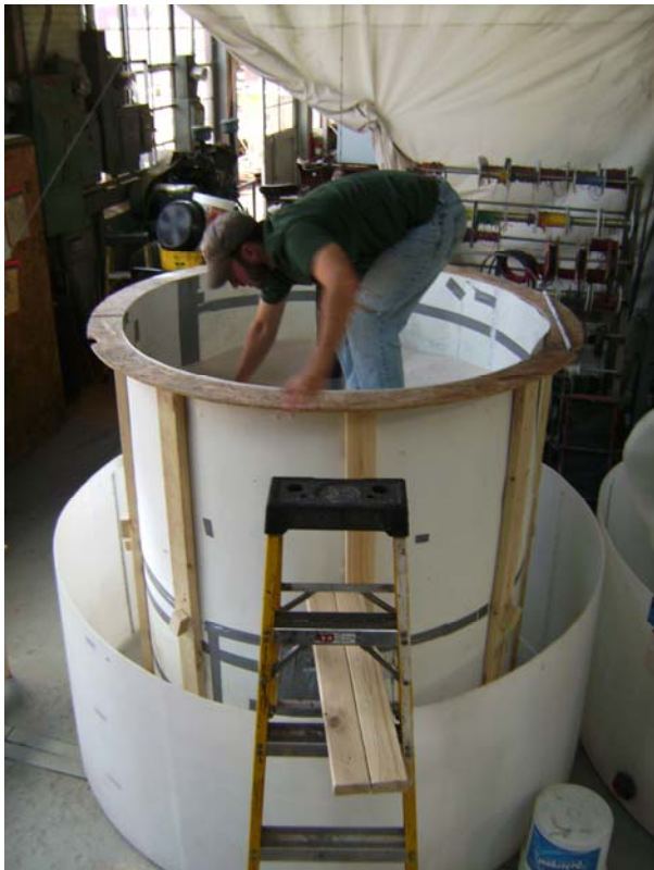
Figure #5: Test tank set up for vertical resolution experiments.
