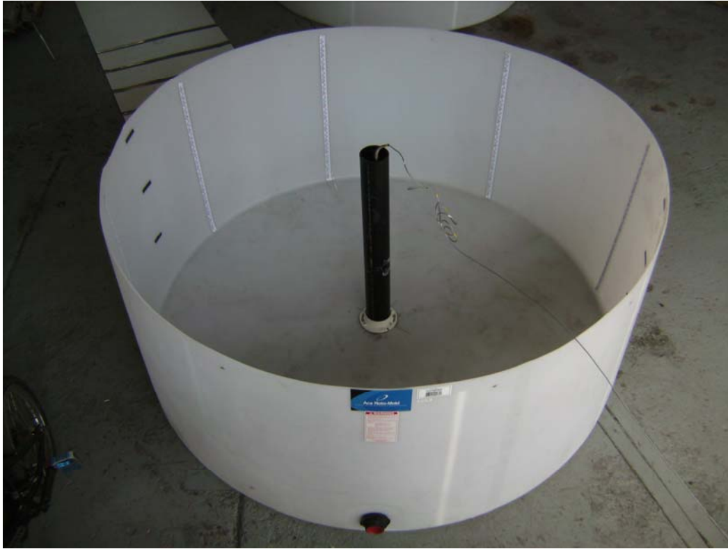
Figure #3A: Empty test tank with 4.5" borehole
